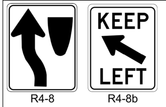
Figure 7. Alternative keep left signs from the Manual on Uniform Traffic Control Devices (MUTCD) .
